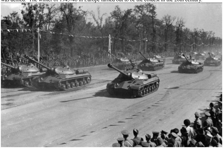
Soviet IS-3 tanks parading on September, 1945 in the Berlin Victory Parade. Its semi-hemispherical cast turret (resembling that of an upturned soup bowl) became the hallmark of post-war Soviet tanks. This Heavy Tank carried a 122 mm gun and had a crew of four.
